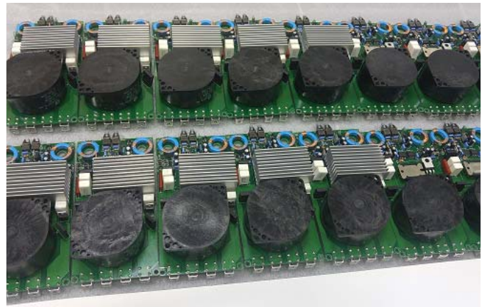
Fig. 8. Constructed storage-switch stage boards with component assembly.
